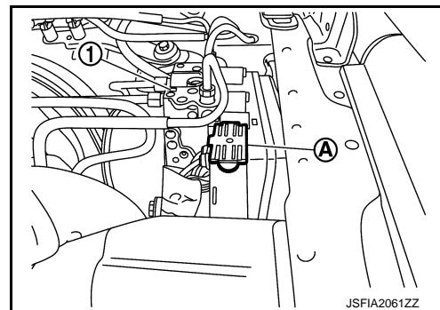
6. Loosen flare nut ① of brake tube ③ using a flare nut wrench, and then remove brake tube from ABS actuator and electric unit (control unit) ②. Refer to [BR-23, "FRONT : Exploded View"](#).
