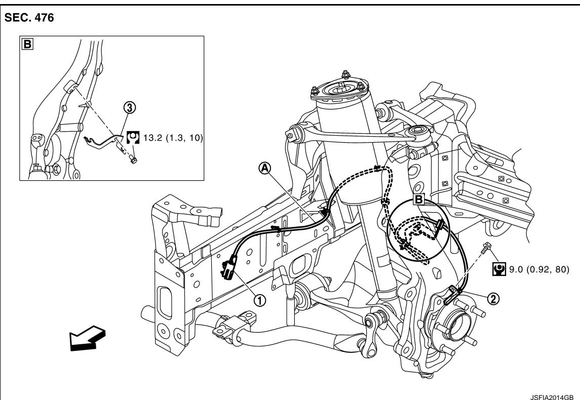
① Front LH wheel sensor harness connector      ② Front LH wheel sensor      ③ Bracket
